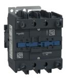
Contactor, TeSys Deca, 4P(2NO+2NC), AC-1, <=440V, 125A, 48V AC 50/60Hz coil, screw clamp terminal
